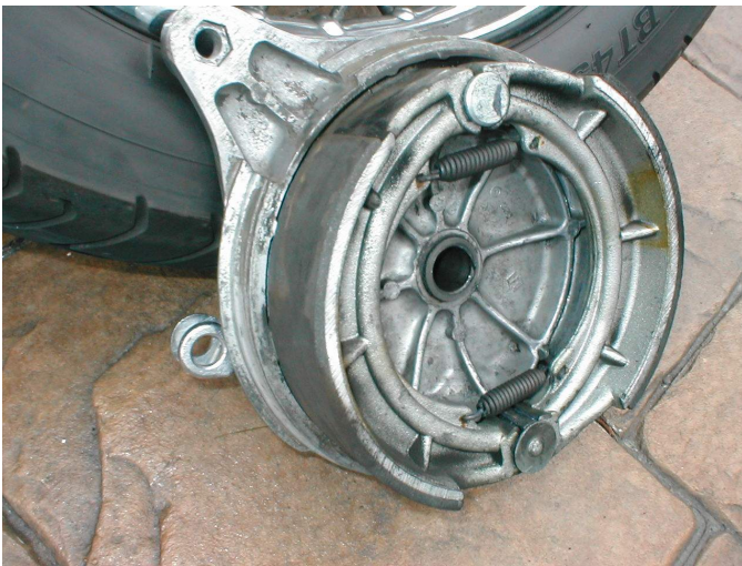
Backplate with brake shoes still in place
